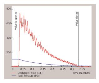
4 A typical air cannon discharge reaches its peak blast force output in the milliseconds just after the valve is opened, dropping quickly as the tank pressure approaches zero
