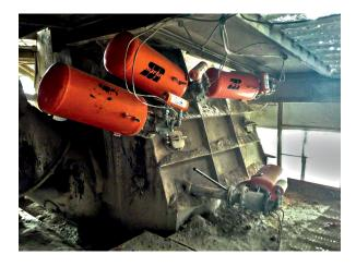
tank is suddenly released by the valve and directed through a nozzle, which is strategically positioned in the tower, duct, cyclone or other location. Often installed in a series and precisely sequenced for maximum effect, the network can be timed to best suit individual process conditions or material characteristics.
